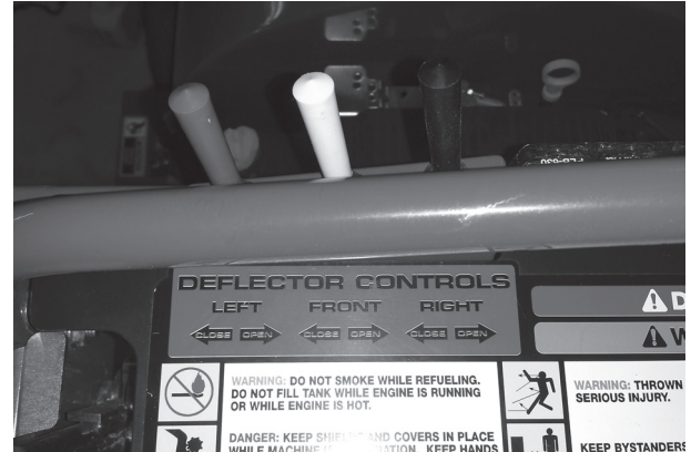
Deflector Control Switches
